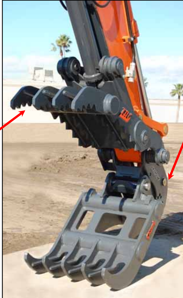
Shown with Hydraulic Pin-Grabber Quick-Coupler and Quick-Link Main-Pin Thumb
