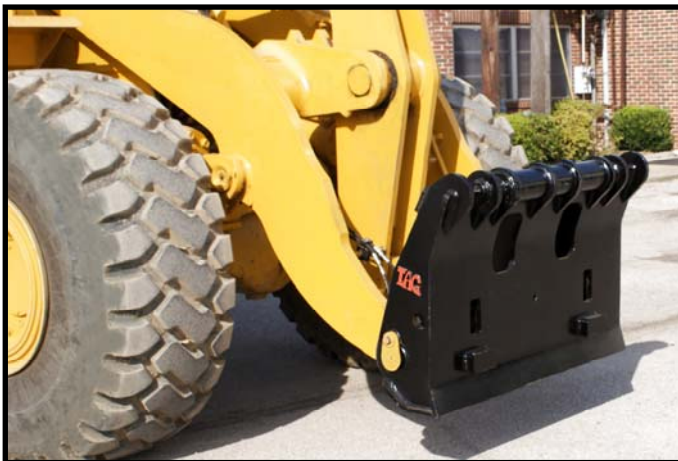
Industry Standard “ JRB “ Style Quick-Coupler with Machine Specific O.E.M. Interface Hydraulic Kits
